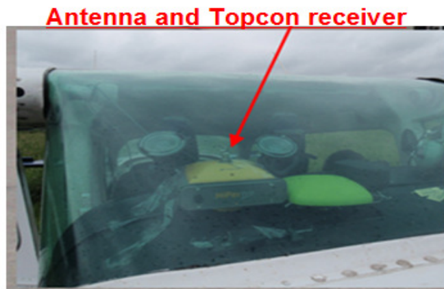
Fig. 1. Antenna and Topcon receiver in pilot's cabin in Cessna 172 plane
